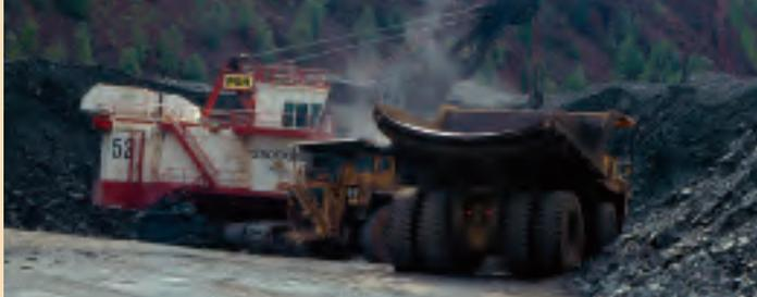
Large amounts of taconite are mined and later crushed to obtain iron ore. An electric shovel (above) loads taconite onto a giant dump truck, which can hold 240 tons of taconite.
